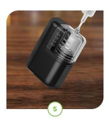
Hold the pump and tubing vertically to ensure any air in the cartridge will be pushed out first. Press and hold the **Pump** button to fill tubing.
