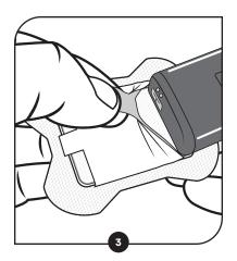
Lift and hold the tab at the end of the sleeve.
