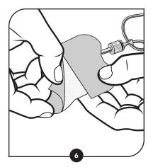
Grip the pump with one hand while you peel off the adhesive paper backing.
