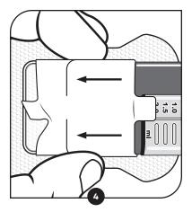
Push the pump through the sleeve until it is fully seated into the tray.
